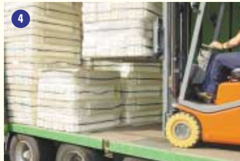
During transportation the load is fixed on the forks.
