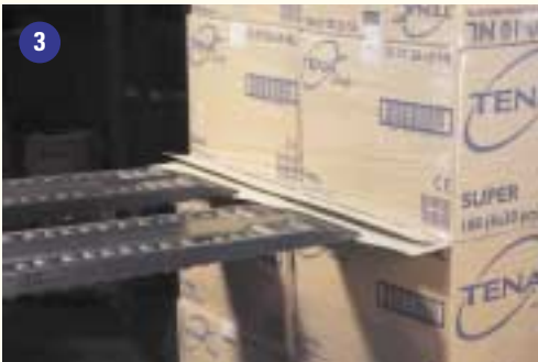
If one load is placed on top of another it is necessary to have them separated by two slip-sheets. The RollerFork® must operate between the two sheets – the bottom sheet allowing the forks rollers to function correctly.
