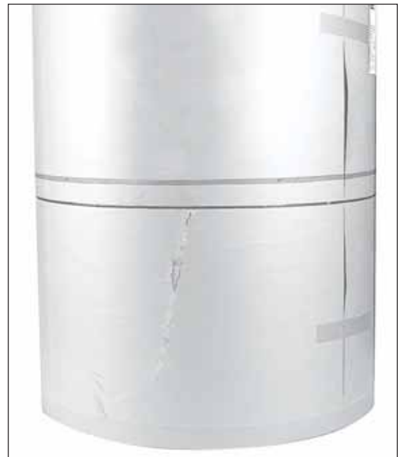
Photo shows damage caused when arm drops due to slack in the chains. This situation can be eliminated with Cascade's Drop Stop Valve. The savings in one day can pay for the added cost.
